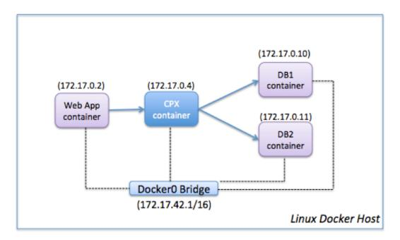
In this example, a web app container (172.17.0.2) is the client and the two database containers, DB1 (172.17.0.10) and DB2 (172.17.0.11), are the servers. The NetScaler CPX container (172.17.0.4) sits between the client and the servers acting as a proxy.
