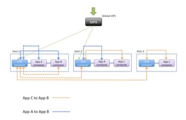
This image shows traffic flow between application C and application B and between application A and application B. When app C (in any of the hosts) sends a request to B, the request is first received on the NetScaler CPX container on the same host as app C. Then, the NetScaler CPX container passes the traffic to the NetScaler CPX container hosted on the same host as app B, and then the traffic is forwarded to app B. A similar traffic path is followed when app A sends request to app B.
