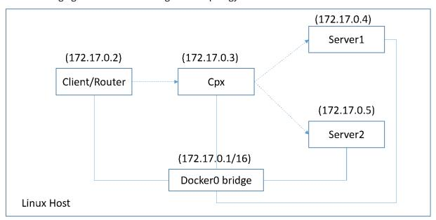
In this topology, virtual servers are configured and advertised (based on the health of services) to the upstream network or router using BGP.
