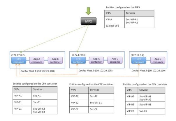
The following table lists the IP addresses and ports that are configured on the NetScaler CPX instances in this example configuration.
