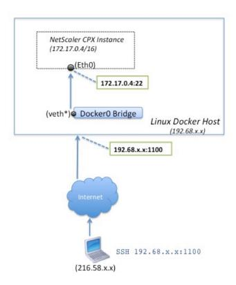
In this example, the Docker host IP address is 192.68.x.x and the single IP address of the NetScaler CPX instance is 172.17.0.4. The SSH port 22 of NetScaler CPX instance is mapped to port 1100 on the Docker host. The SSH request from the client is received on IP address 192.68.x.x at port 1100. The Docker host performs port address translation to map this address and port to the single IP address 172.17.0.4 on port 22 and forwards the client request.
