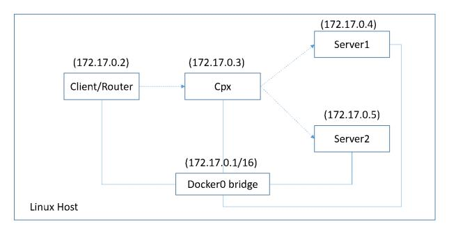
In this topology, virtual servers are configured and advertised (based on the health of services) to the upstream network or router using BGP.
