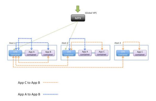
This image shows traffic flow between application C and application B and between application A and application B. When app C (in any of the hosts) sends a request to B, the request is first received on
