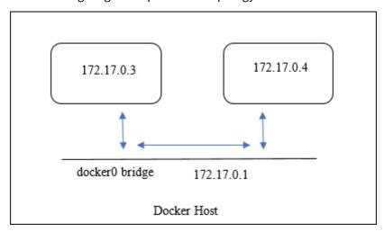
In this example two NetScaler CPX instances, CPX-1 (NSIP: 172.17.0.3) and CPX-2 (NSIP: 172.17.0.4), are created on the same Docker host. For high availability support, you must configure high availability nodes on both NetScaler CPX instances using the NSIP of the other node.
