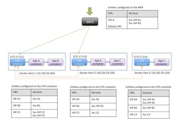
The following table lists the IP addresses and ports that are configured on the NetScaler CPX instances in this example configuration.
