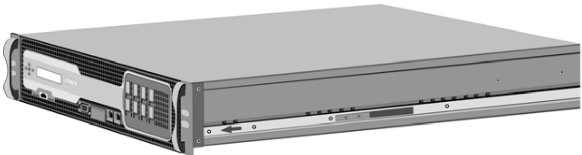
Figure 1. Attaching inner rails
