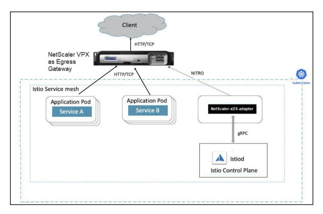
For detailed instructions on how to deploy NetScaler VPX as an Egress Gateway, see Deploying NetScaler with Istio.
