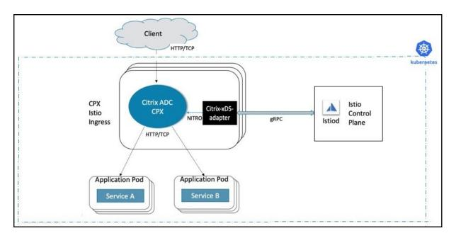
For detailed instructions on how to deploy NetScaler CPX as an Ingress Gateway, see Deploying NetScaler with Istio.
