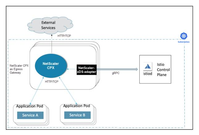
For detailed instructions on how to deploy NetScaler CPX as an Egress Gateway, see Deploying NetScaler with Istio.
